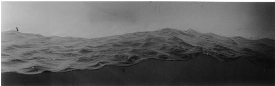
FIGURE 3. Photograph of the tank surface at a location between probes 6 and 7 for paddle waves of f_p = 1.11 Hz, ak_0 = 0.19 exposed to a wind in the upper cavity of U_{cl} = 7 m s ^{-1} . Note the presence of microscale waves over the entire wave surface with steeper waves on the crest of the lower-frequency paddle wave. The low-frequency paddle wave is travelling from left to right and the wind is from right to left.
